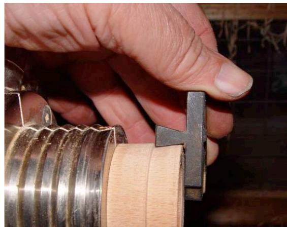
This simple device obviates the need for callipers and enables me quickly to zip a spigot down to size, simultaneously checking the angle by comparison, without fear of going under size by accident.
