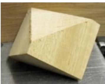
After three or four efforts with varying degrees of success I thought that instead of sanding the flats for the centres it would be better if I sawed off the corners to form a much bigger triangle to save a lot of turning time and effort. The corners could be cut down to a size closer to the diameter of the spigot which forms the base. (As it happened the sawn off pyramids eventually made quite neat little desk pen holders – at the suggestion of my youngest granddaughter). Problem:
