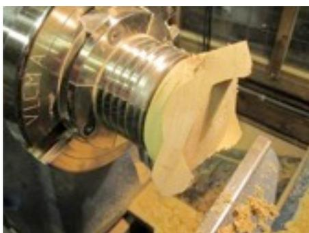
to have maximum revs on for this job because then the sanding disc, being, as it is, in a hand held drill, does not get time to drop into the gaps. I also think that turning at high speed with a very sharp tool reduces the amount of break out on the end grain when air turning is involved. I expect this idea to be frowned upon by the pundits but you can do what you like when nobody is watching can't you? I also like to do it with the lathe in reverse.
