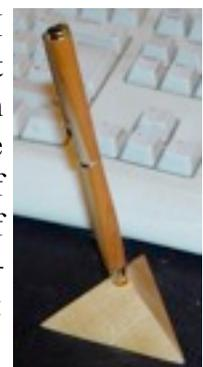
How do you hold a cube in order to cut an accurate three sided pyramid off a corner? If you have the time to spare stop here; pick up a box of some sort and think about it. I made a jig to hold the cube at 45 degrees to the saw blade in two planes. This worked after a fashion but did not produce the isosceles triangle shape.
